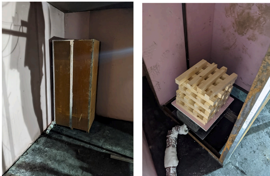
Fig. 7. Simulated fridge in the corner of the room (left) and load cell loaded with Fuel Package I (right).
