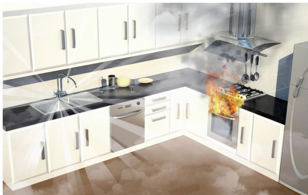
buildings and ... fit for their intended purpose”<sup>3</sup>. An example is Automist, a high-pressure mist device which mounts around the kitchen sink or on a wall. In the event of a fire, a heat alarm activates at 57°C and a high pressure pump powers just 5lpm of fine water mist throughout the volume to be protected. This allows fire suppression coverage to be retrofitted to a targeted area, for example an open plan lounge.
